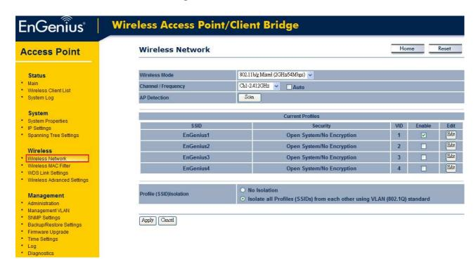
3. To configure Wireless VLAN Tagging, please press Edit at Wireless Network section.
